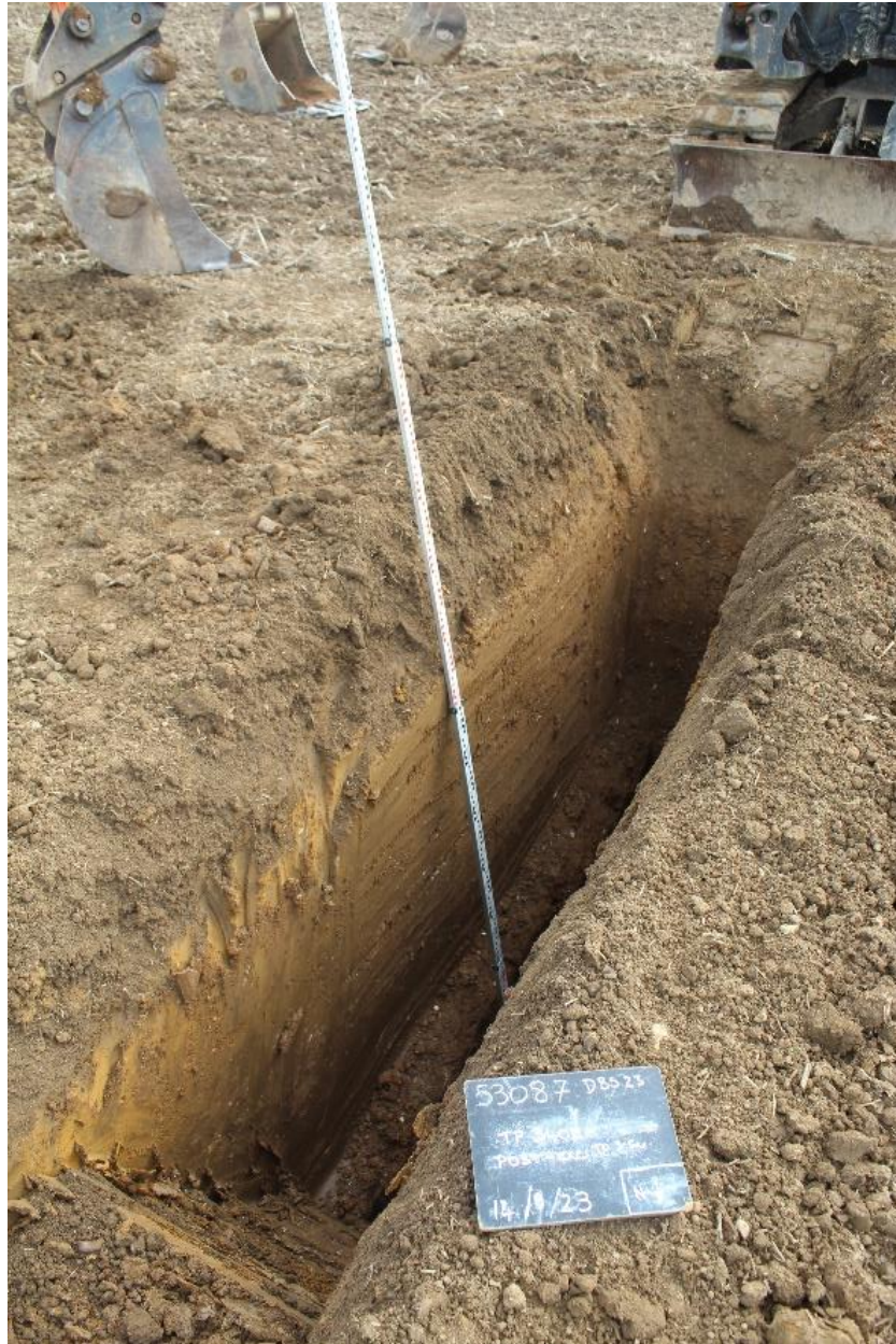
Plate 6: Test pit [3405] excavated to 3.5m, viewed from the south-east.
